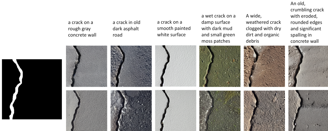
Figure 10: Text-prompt control in background-free mode. All images are generated from the mask on the left. Each column corresponds to one text prompt, and the two rows show two samples per prompt.
