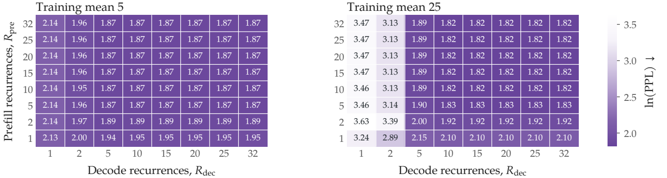
Figure 11: Prefill gains saturate by R_{\text{pre}} = 5 , and decode depth matters more. Cells give the cached log-perplexity of Small checkpoints trained at mean recurrence 5 (left) and 25 (right), on CacheEval with terminal KV sharing, 1,024 prefix tokens, and continuation positions 2–512.
