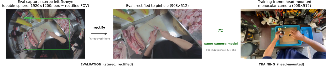
Figure 13: Rectifying the evaluation set onto the training camera model. Left: the raw capture from the stereo rig’s left camera, a wide-angle double-sphere fisheye ( 1920 \times 1200 ); the green box marks the region that maps into the rectified image. Middle: that region undistorted to a 908 \times 512 pinhole. Right: a training frame, shown for comparison.
