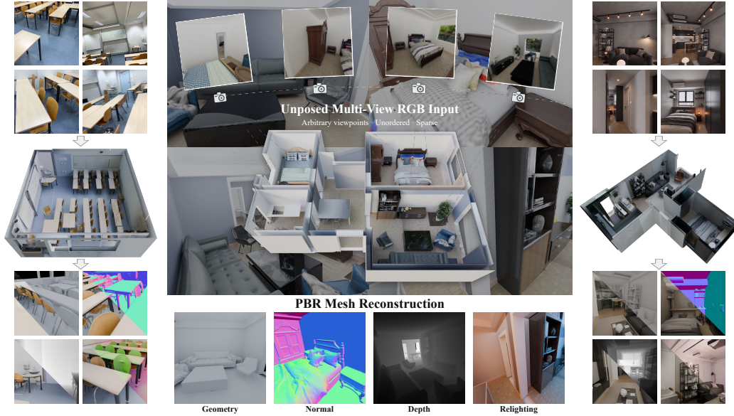
Figure 1: WorldRecon Overview. Given unposed multi-view RGB images of an indoor scene, WorldRecon reconstructs a complete scene-scale PBR mesh block-by-block via a native 3D generative prior at arbitrary scene scales, yielding high-fidelity geometry, depth, normal, and texture. From left to right, we demonstrate WorldRecon on real-world captures, synthetic images, and frames from generated videos, highlighting generalization across diverse input domains.
