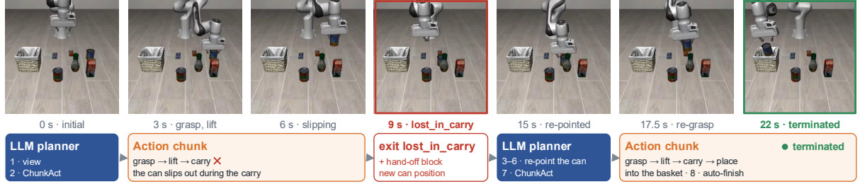
Figure 4: Demo of a successful rollout on LIBERO-Pro with ChunkAct. Given the task “pick up the can and place it in the basket,” the LLM planner first perceives the scene and invokes ChunkAct to execute a chained action sequence. The can is grasped successfully but slips during transport, so ChunkAct returns the error code. The planner interprets this feedback, re-localizes the can, and invokes ChunkAct again, which completes the task.
