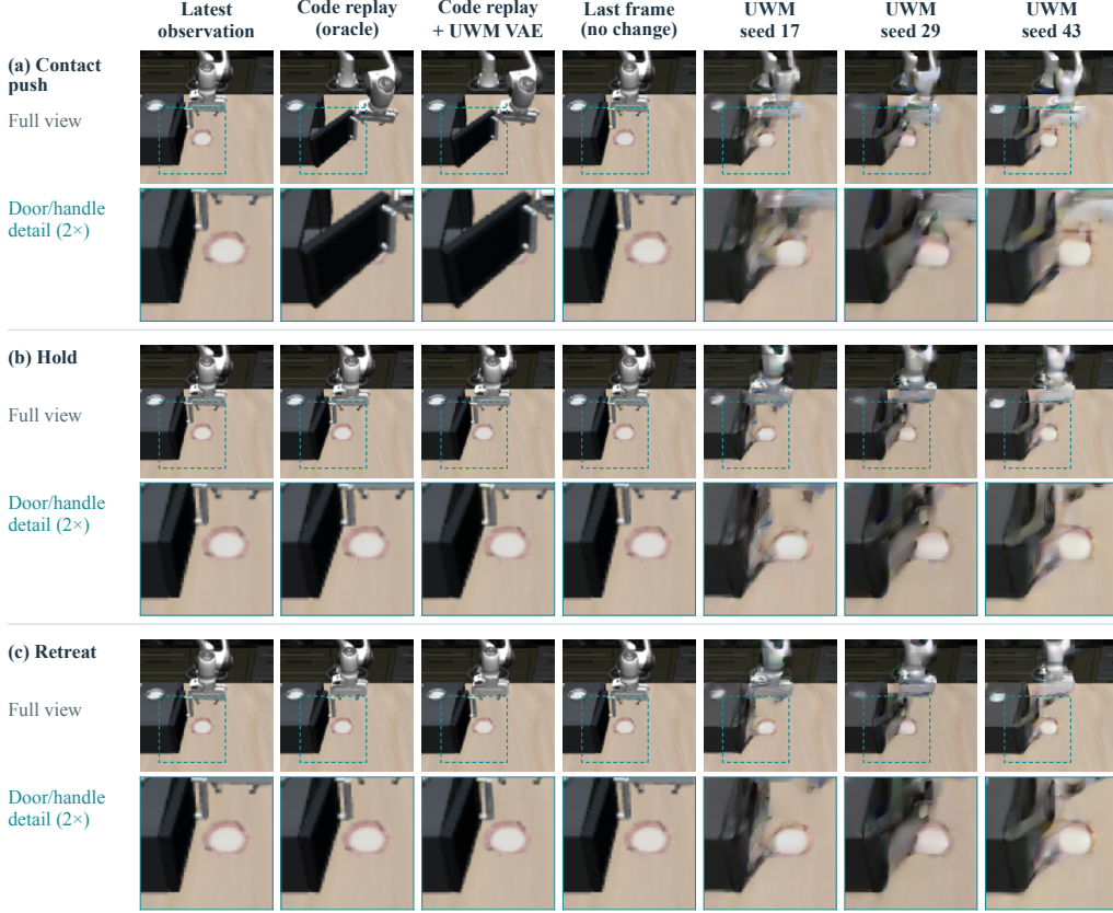
Figure 15: Articulated code simulation vs. UWM rollouts on the generated asset (Initial State 1). Rows correspond to contact push, hold, and retreat control sequences (16 commands at 20 Hz). Columns show the initial observation, MuJoCo simulation of the generated 3D code, its reconstruction through UWM’s frozen VAE, the static last-frame reference, and all three UWM rollout seeds. Enlarged 2 \times crops (dashed boxes) demonstrate that executable 3D code preserves sharp, consistent door and handle geometry both before and after VAE reconstruction, whereas UWM rollouts exhibit seed-dependent contour drift.
