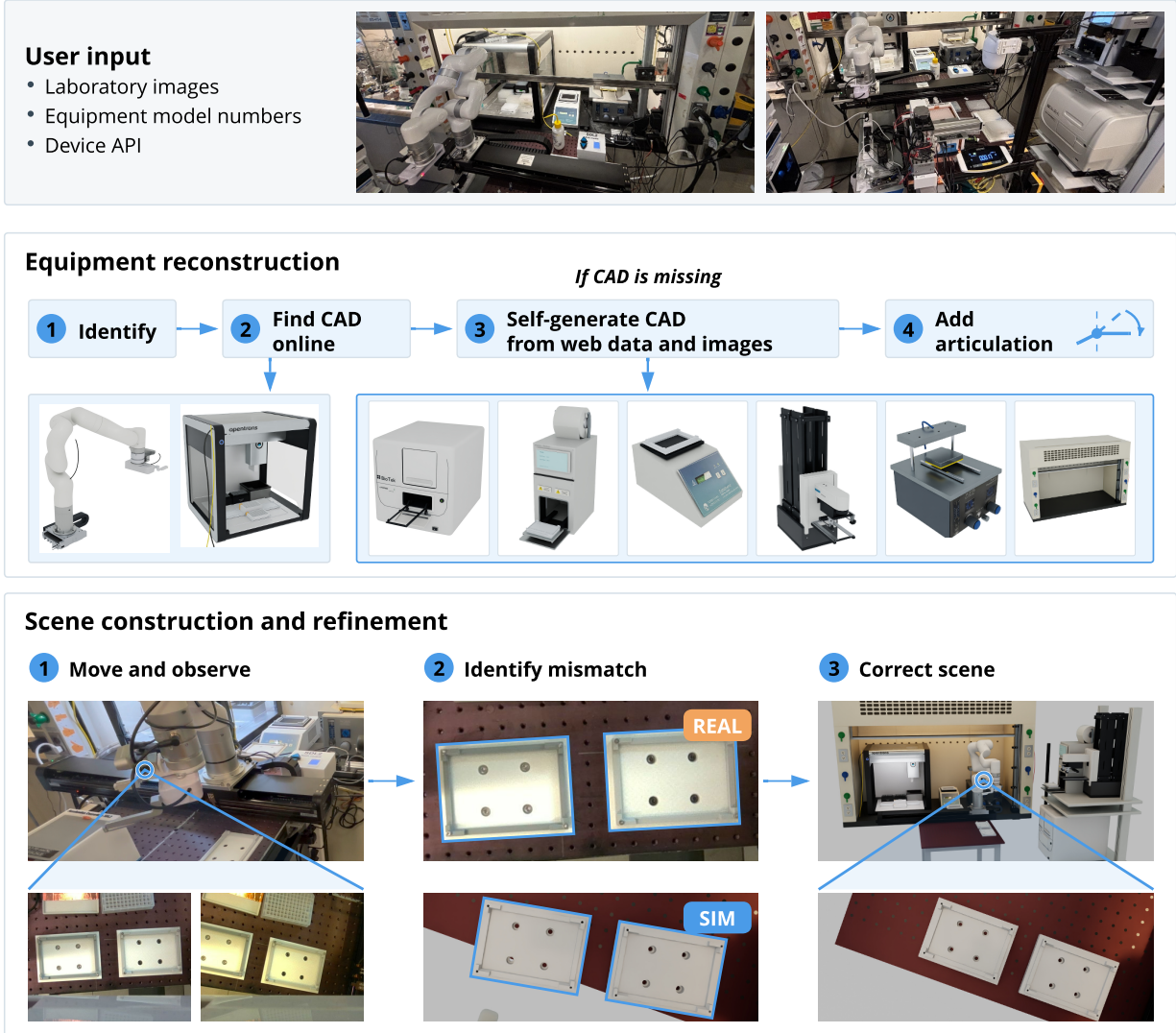
Figure 3 Building a digital twin of the laboratory. (a) Starting from laboratory images and equipment model numbers when available, the twin agent identifies individual devices, searches product documentation, and retrieves or constructs equipment models with task-relevant geometry, articulation, and control interfaces. (b) These models are assembled into an initial simulation scene and refined using colour and depth observations acquired from multiple robot poses. The agent compares observed and rendered views and iteratively updates equipment poses to align the scene with the physical laboratory.
