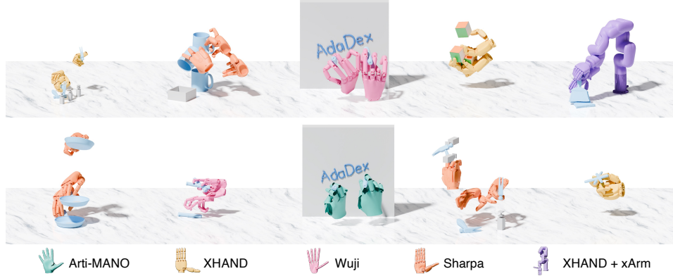
Figure 5: ADaDEX learns diverse skills such as functional grasping, in-hand reorientation, dynamic throw-and-catch, and can achieve various downstream tasks with high dexterity. Our method also works on various robot hand embodiments and real arm-hand systems.
