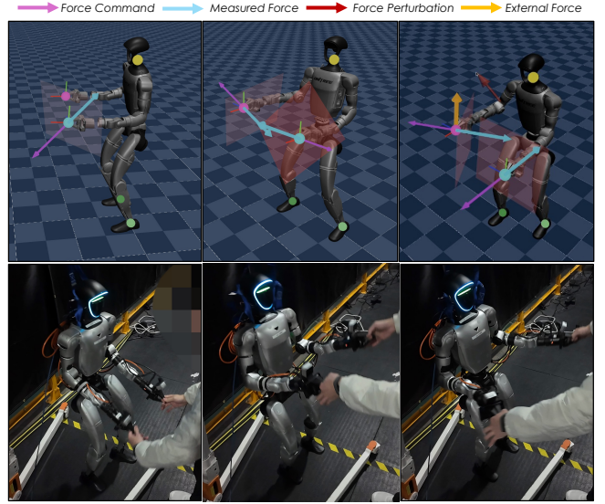
Fig. 5. Hybrid compliance whole-body controller with force tracking. Top: in simulation, each hand presses a randomly placed virtual plane while the robot tracks the reference motion and maintains balance. The arrows show commanded force (pink), measured reaction force (blue), external force (yellow), and force perturbation (red). Bottom: on the real robot, a person pulls both hands, which yield instead of resisting.
