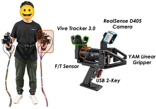
Fig. 4. Robot-free data-collection interface. Left: the demonstrator holds a handheld device in each hand and wears trackers on the chest and both ankles. Right: each device carries a VIVE tracker, a RealSense D405 wrist camera, and an F/T sensor mounted between the handle and gripper.
