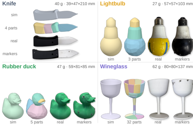
Fig. 3: Objects used in our experiments. For each object we show its simulation mesh, its collision meshes from convex decomposition, the real object, and the real object with motion-capture markers.
